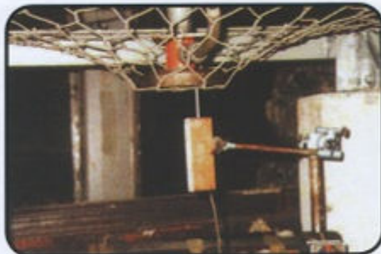
Deformation of panel during loading
