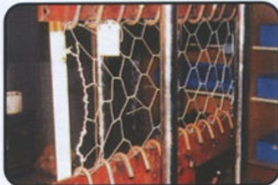
Tensile Test In Air (perpendicular to the direction of twist)
