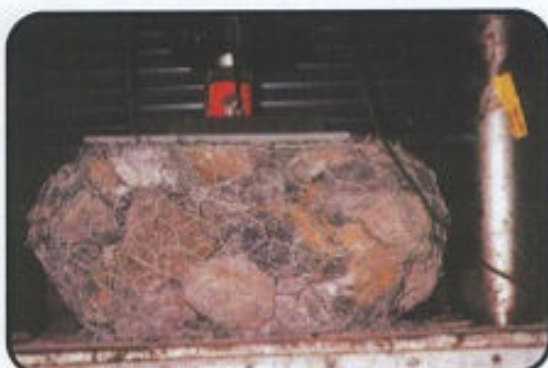
Compression test on rockfilled gabion
